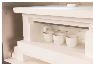
Picture 2 Milestone PYRO Sulfated Ashing muffle system
