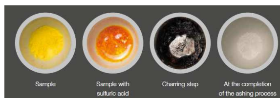
Picture 3- Samples during the steps of sulphate ashing run
